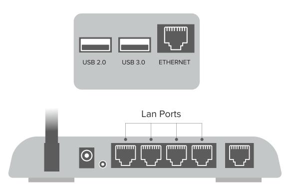
2. Plug the Main Hard Disk to USB2 and Backup Hard Disk to USB1. Keep the Hard Disk in Hard Disk tray.
